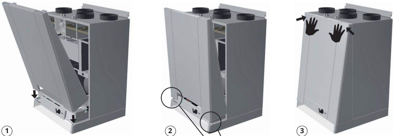
1. Lower the front edge of the door into the leading edge of the unit.
