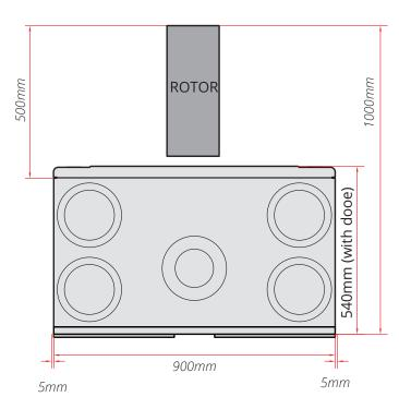
NB! The door of the unit is too heavy to hold itself closed when the unit is on the floor. It must therefore be secured with two end studs and a strap.
