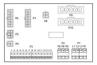
It is a circuit board that distributes the power supply to the components of the ventilation unit (not the electric heating coil) and control cabinet. There is also a terminal block for the components required to regulate a water heating coil.
