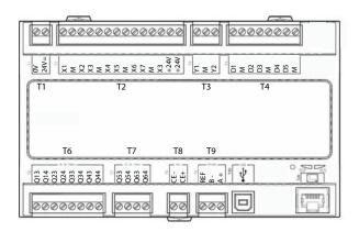
The ventilation unit's control unit This is where the control panel (HMI) and sensors and other components of the ventilation unit are connected. It is also possible to connect an SD memory card to back up or reload configuration settings and parameters for the system.
