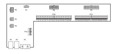
It is a circuit board that connects the components to the control unit. External components such as dampers are connected to this board via the terminal blocks on the board.
