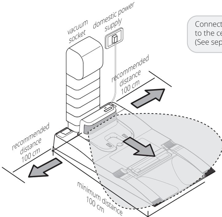
Connect the docking station to the central vacuum unit. (See separate manual).
