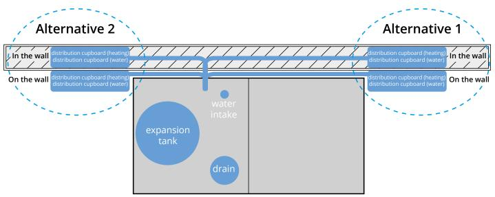
The product must be connected to a drain It is recommended that the drain is located near to or under the product (see sketch)
